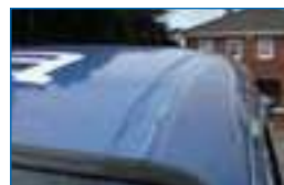
Due to the silicone content in modern car lacquers the adhesion of can be far from optimal. under tension (especially in recesses) is bound to come loose and ultimately be returned for repair or renewal.
